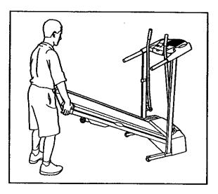
2. Move your right hand to the position shown and hold the treadmill firmly. Press out on the storage latch. Raise the treadmill until the storage latch closes over the catch. Make sure that the storage latch is fully closed over the catch.
